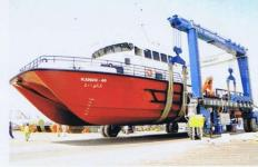
draught of 1.2 metres. Built under survey to Bureau Veritas, the crew boat has a deck cargo capacity of 35 square metres and can carry a crew of 5 and up to 35 passengers.
