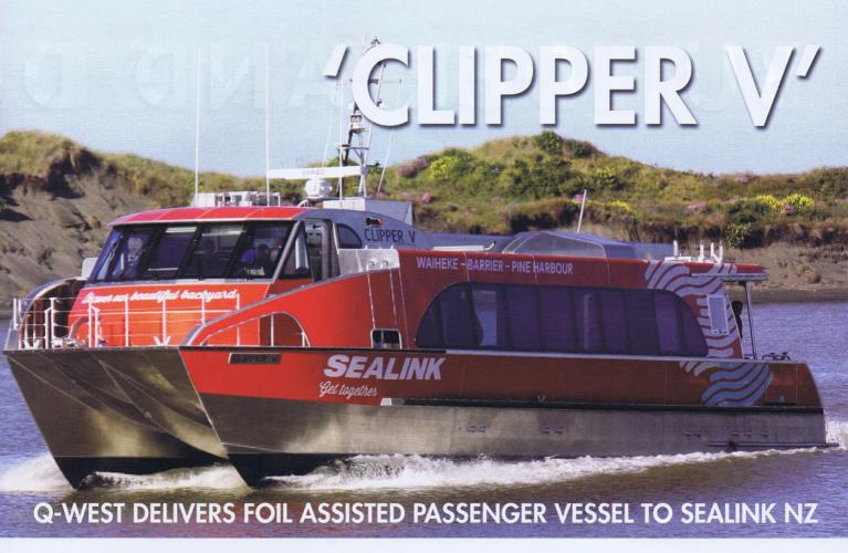
Q-West Boat Builders of New Zealand has teamed up with Teknicraft to complete a fifth foil assisted passenger vessel for Sealink NZ. The first in the series was a 12-metre, the second and third were 16 metres and the fourth was 17.5 metres.
